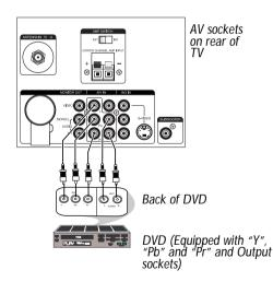
You can view the playback of DVD discs by using the COMPONENT VIDEO INPUT sockets on the rear of the TV.
